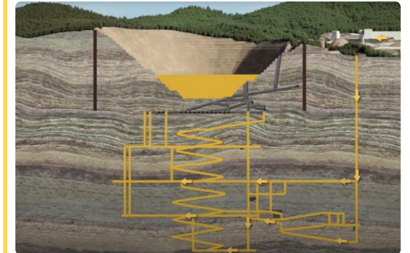
Tailings used as paste back-fill
