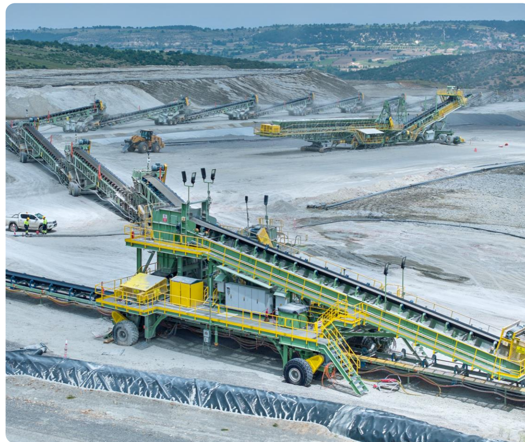
Grasshopper conveyors delivering material to the leach pads.
